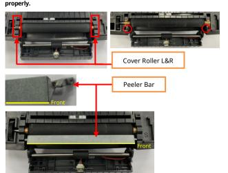
9. Reinstall the Cover Dip that was removed in step 7. Then, connect the power supply and turn the power on to check if the Peeler Sensor LED is green when turned on.
