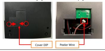
8. Insert the Peeler Wire to the Peeler Connector (yellow square) in the correct direction.
